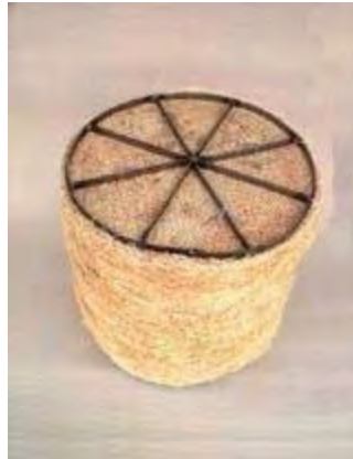
Figure 3: Coalescing “Hay Pack” constructed of excelsior wood shavings. (Note: Shown placed on end: support wheel on end would be vertical when installed)
