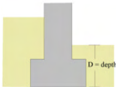
Figure 3 – Depth of Footing
