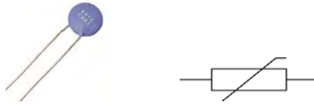
Figure No. 8 – Thermistor and Its Electrical Symbol
